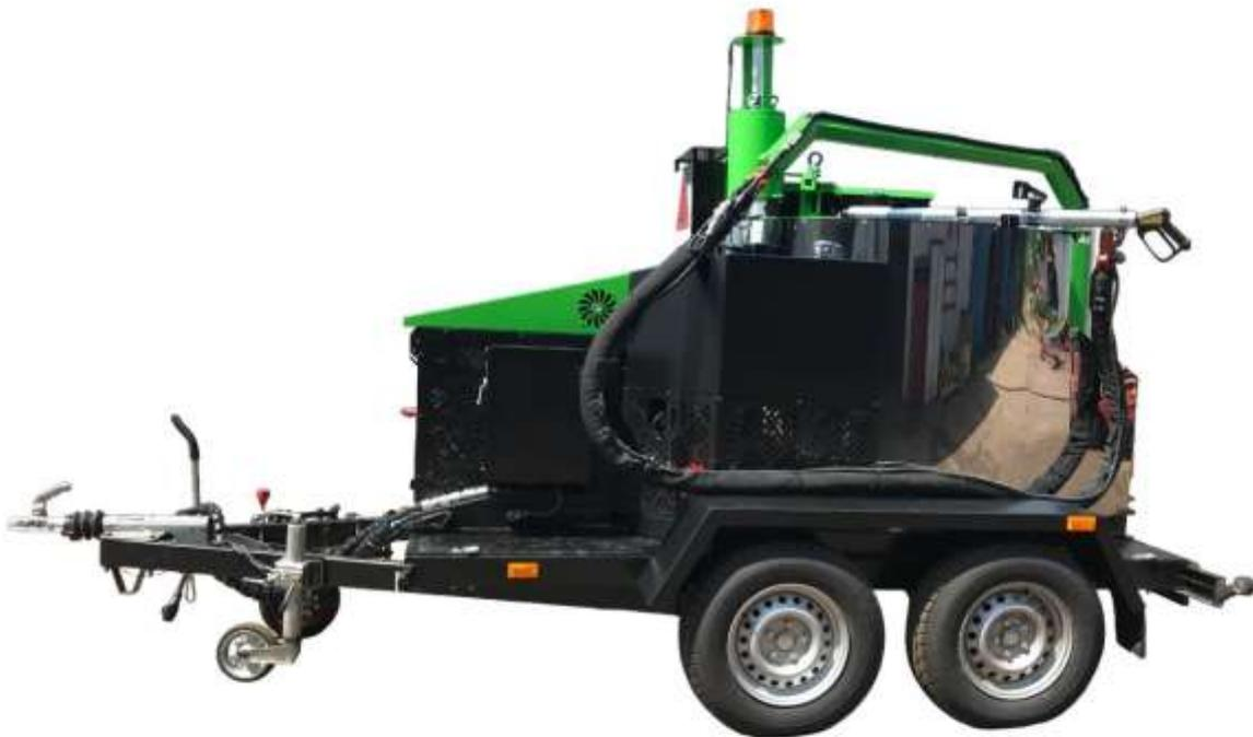
Crack sealing machine BPM-500 is used for sealing cracks, seams and waterproofing, as well as for repair and construction works on roads with the use of bitumen-elastomeric sealing mastic. Specially designed sleeve fastening system, which significantly reduces the likelihood of its failure.
